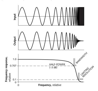
Loosely speaking, *bandwidth* is the rate at which information in a signal can change from one state to another. The response of an electronic system deteriorates above a certain information rate. Bandwidth is specified or measured at the frequency where amplitude has fallen 3 dB from its value at zero frequency (called DC) – that is, to the fraction 0.707 of its value at DC.
