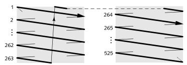
Figure 1.7 exaggerates the slant of a fraction of a degree that results when a conventional CRT – either a camera tube or a display tube – is scanned with analog circuits. The slant is a real effect in analog cameras and displays, although it is disregarded in the design of equipment.
