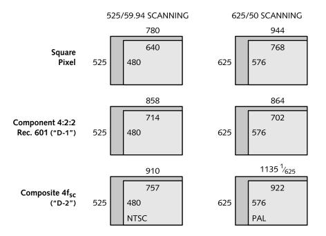
Figure 1.5 **Digital video rasters.** The left column shows 525/59.94 scanning, the right column shows 625/50. The top row shows sampling with square pixels. The middle row shows sampling at the Rec. 601 standard sampling frequency of 13.5 MHz. The bottom row shows sampling at four times the color subcarrier. Blanking intervals are shown with dark shading.
